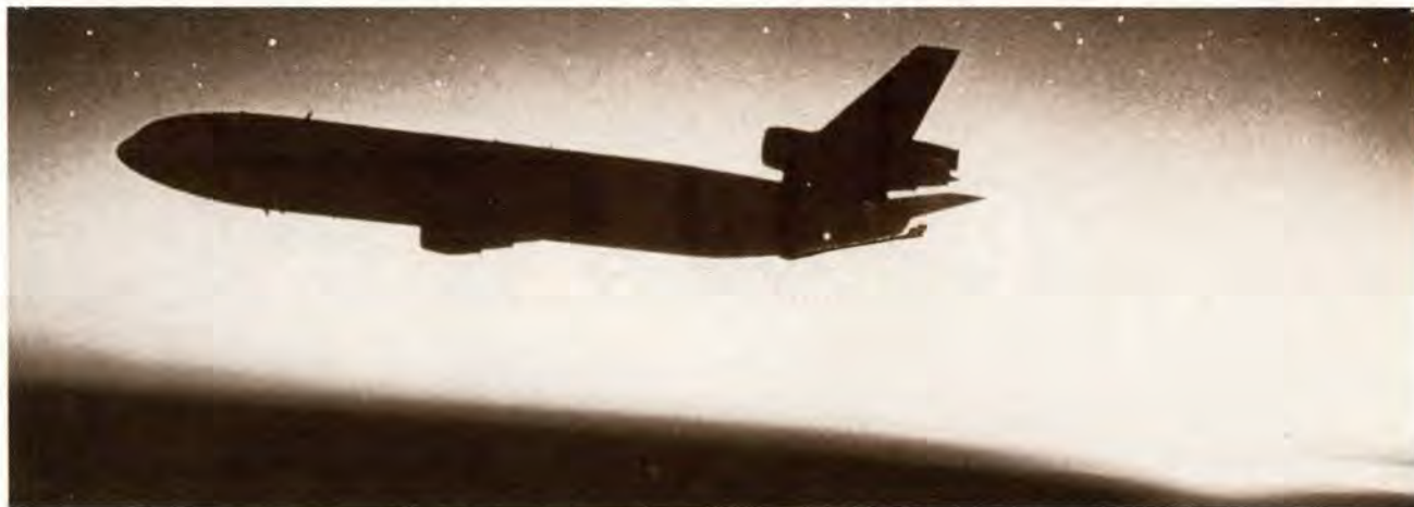
Fully loaded, the KC-10 carries more than 356,000 pounds of fuel, almost twice as much as the KC-135. Air refueling one of these 590,000-pound leviathans at night is a demanding task for any pilot. Teaching a new AC requires special techniques and a lot of patience.
